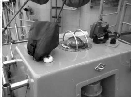
Figure 9. DF Display Hood – display covered
