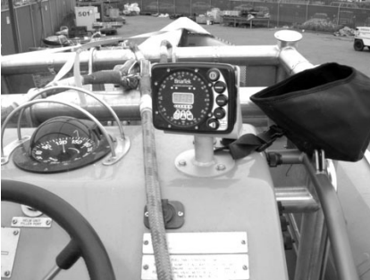
Figure 8. DF Display Hood – display uncovered
