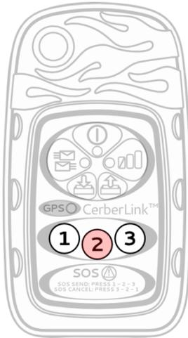
A breadcrumb is a single GPS coordinate and time stamp that can be viewed on the CerberCenter website or shared on your Public Activity page. You can send a breadcrumb directly from CerberLink using the keystroke **2-2-2** on the keypad. This will create a breadcrumb message containing the current location and will automatically perform a mailbox check.
