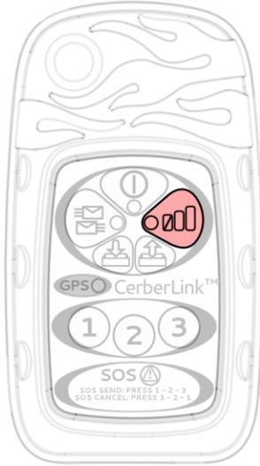
Press the signal strength button to check for satellite signal strength. For best signal, find a clear view of the sky and orient the device upright. The status light stays OFF until a signal strength is calculated; this may take up to 1 minute. Signal strength is indicated as shown below. Iridium satellites pass overhead quickly; so short periods with no signal are common. Keep this in mind when using this feature.
