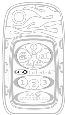
The GPS indicator shows the status of CerberLink’s internal GPS. When the indicator is flashing green, CerberLink has adequate GPS signal. When the indicator slowly flashes red, CerberLink is unable to attain a strong enough signal to record position data.
