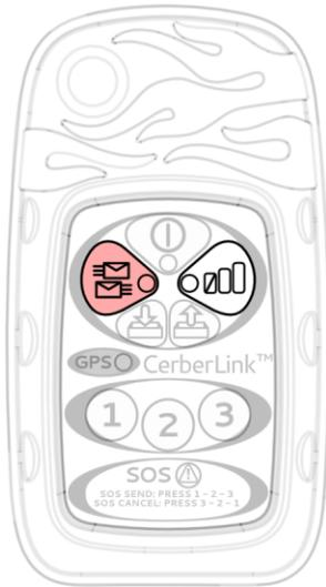
Press the mailbox check button to send and retrieve messages via satellite. A mailbox check will send any stored messages and/or tracks in CerberLink’s outbox and will save any newly received messages from the satellite network in its inbox. The progress of the mailbox check can be viewed on the status light. The mailbox check LED will flash rapidly until **all** messages have been transferred to/from CerberLink while it communicates with a satellite.
