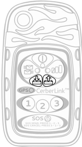
These indicators show the status of the CerberLink inbox and outbox. Messages sent to CerberLink via the CerberTouch app appear in the outbox. New messages received via satellite will appear in the inbox. To read new messages residing in CerberLink's inbox, press the "Sync" button in the CerberTouch app. This will initiate a Bluetooth transfer of all new messages to the CerberTouch app. See **sect. 7.6**, Sync and Mailbox Check for additional information.
